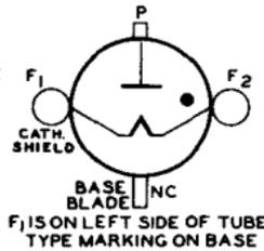
F1 - Filament, Cathode Shield (Anode Return)
