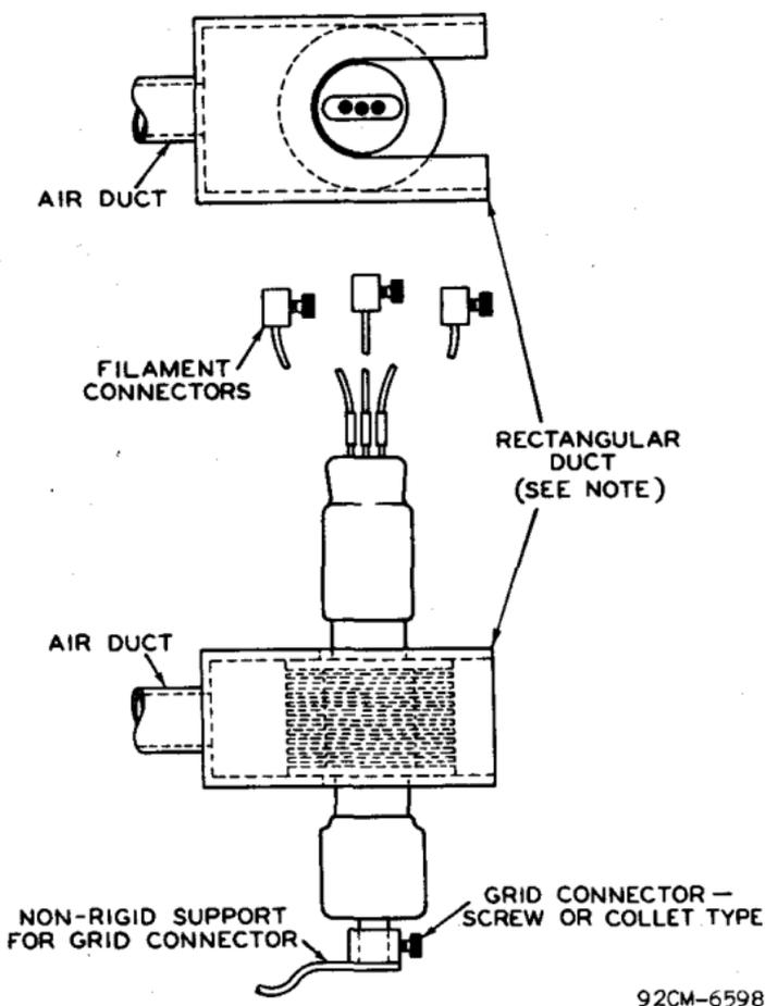
NOTE: AIR DUCT MAY BE PART OF HIGH-FREQUENCY TRANSMISSION LINE. UPPER AND LOWER FACES OF RECTANGULAR DUCT HAVE SLOTS TO PERMIT PASSAGE OF TUBE. MEANS SHOULD BE PROVIDED TO LOCK TUBE IN POSITION.
