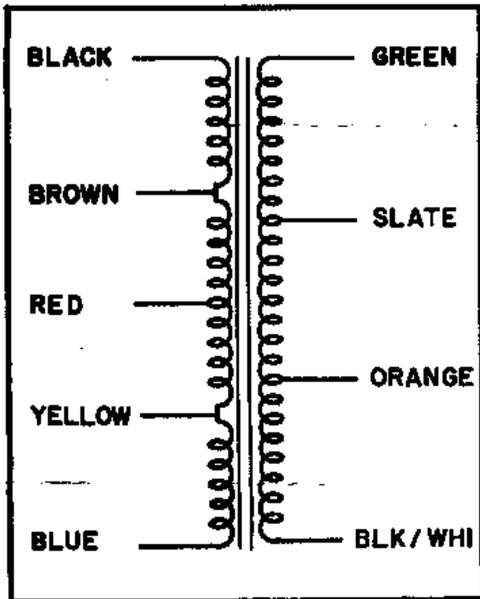
Primary 8,800 Ohms CT at 100 MADC each side of CT. Provided with screen taps for Ultra-Linear operation. Connect Black to the Plate and Brown to the screen of one of the Push-Pull output tubes. Connect Blue to the Plate and Yellow to the screen of the other Push-Pull tube. Red connects to B(Plus).
