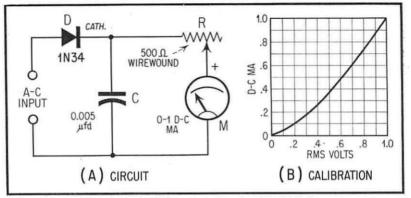
Fig. 2. Diode-Milliammeter Circuit with Multiplier.
