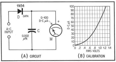
Fig. 3. Series Diode-Microammeter Circuit.
