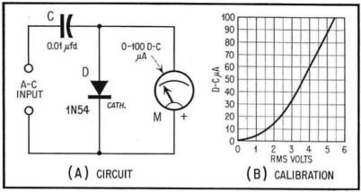
Fig. 4. Shunt Diode-Microammeter Circuit.
