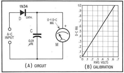
Fig. 1. Basic Single-Diode Circuit with Milliammeter.
