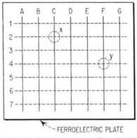
Arrangement of Ferroelectric Fig. 5. Memory.
