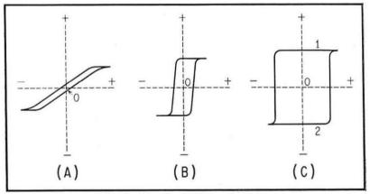
Fig. 4. Ferroelectric Hysteresis Loops.
