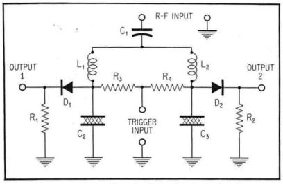
Fig. 6. Ferroresonant Circuit Employing Ferroelectric Capacitors.
