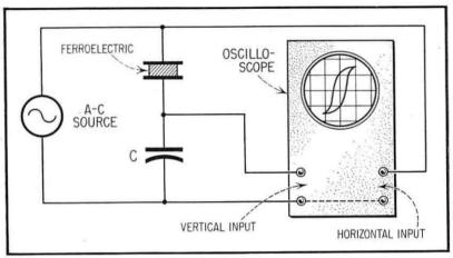
Fig. 3. Setup for Checking Ferroelectric Hysteresis.
