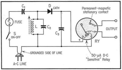
Fig. 3. Diode-Type Wired-Radio Receiver.
