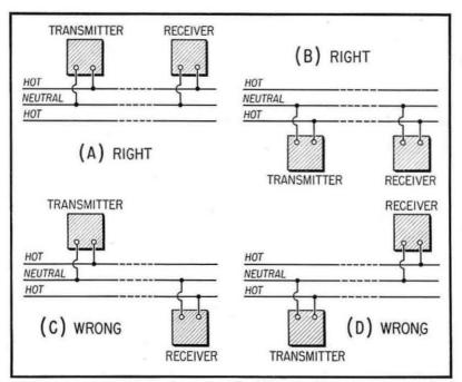
Fig. 5. Connections To 3-Wire Service.
