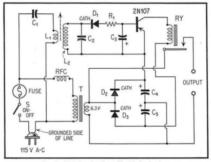
Fig. 4. Diode-Transistor-Type Wired-Radio Receiver.
