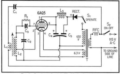
Fig. 1. Transformer-Coupled Wired-Radio Transmitter.
