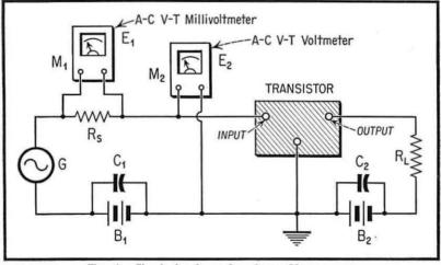
Fig. 4. Circuit for Input Impedance Measurement.
