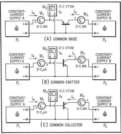
Fig. 2. Setups for Checking R<sub>11</sub> and R<sub>12</sub>.
