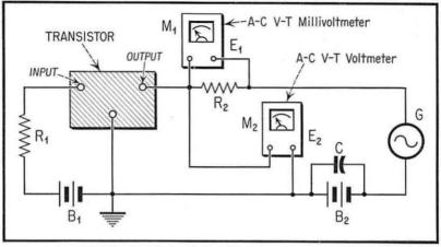
Fig. 5. Circuit for Output Impedance Measurement.
