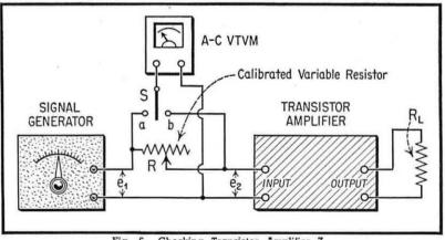
Fig. 6. Checking Transistor Amplifier Z.
