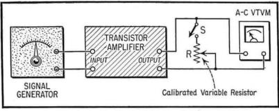
Fig. 7. Checking Transistor Amplifier Z.
