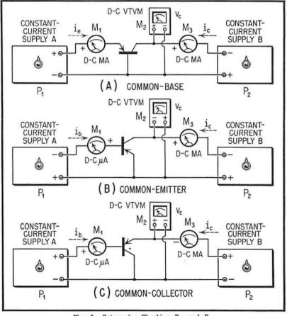
Fig. 3. Setups for Checking R, and R,
