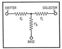
Fig. 1. Simplified 3-Terminal Equivalent of Transistor.
